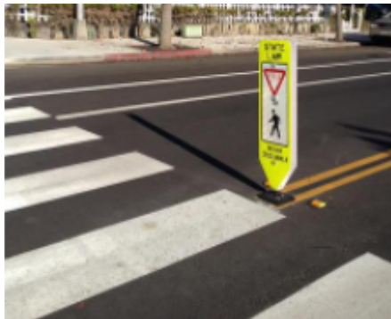
In-Street Pedestrian Signs: gives drivers additional reminder about pedestrians, and slows drivers down Cost: Low
